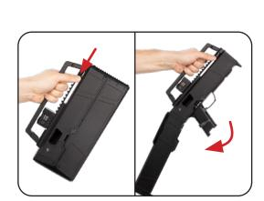
3. Push out the disassembly pin from the left to right. The pin is captured and will not detatch completly.
